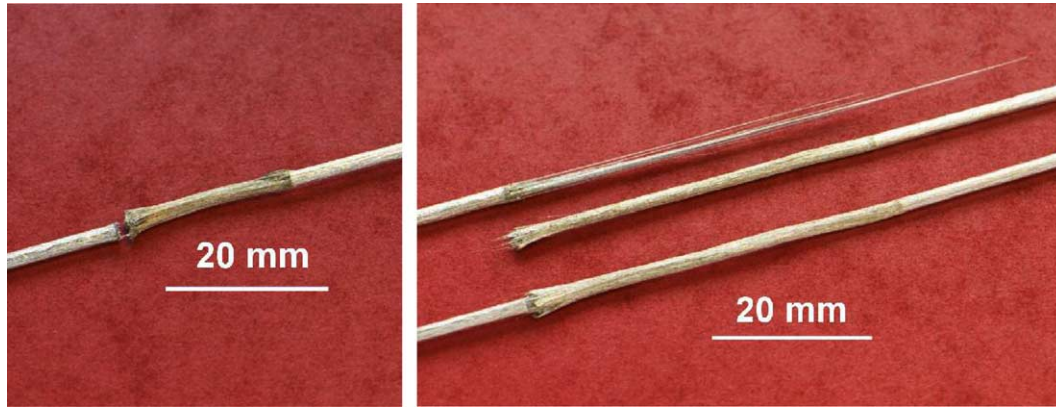
Fig. 7. Left: macroscopic failure at the solid/liquid transition for specimens with a molten length l \leq 50 mm. Right: two specimens with l > 50 mm after failure (i.e. strained beyond the peak stress); the lower specimen is as-retrieved from the tensile testing apparatus, the upper specimen was pulled apart while molten until full separation in two halves.
