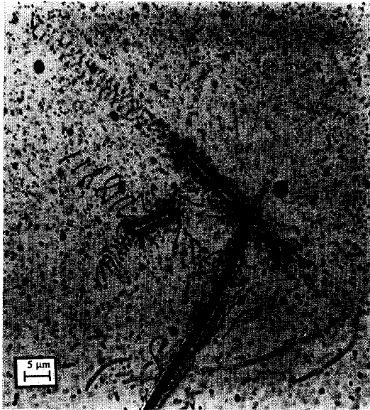
Fig. 13. Three glass fibers having emitted decorated dislocations in AgCl. Fiber A punched a row of loops at each of its end. Fiber B punched four rows, two of which are blocked by fiber A and C. Fiber C is surrounded by a plastic zone in which some dislocations can be resolved.
