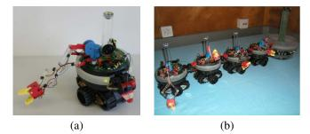
Fig. 1. The swarm-bot concept: (a) a mobile module called *s-bot*, fully autonomous in perception, control, action, and power, capable of approaching and assembling with its teammates, (b) a modular robot called *swarm-bot*, composed of four s-bots, manipulating an object.
