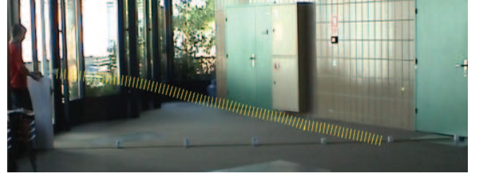
Fig. 9. Flight trajectory, launching velocity 2m/sec and launching angle \gamma \approx 3.5^\circ .
