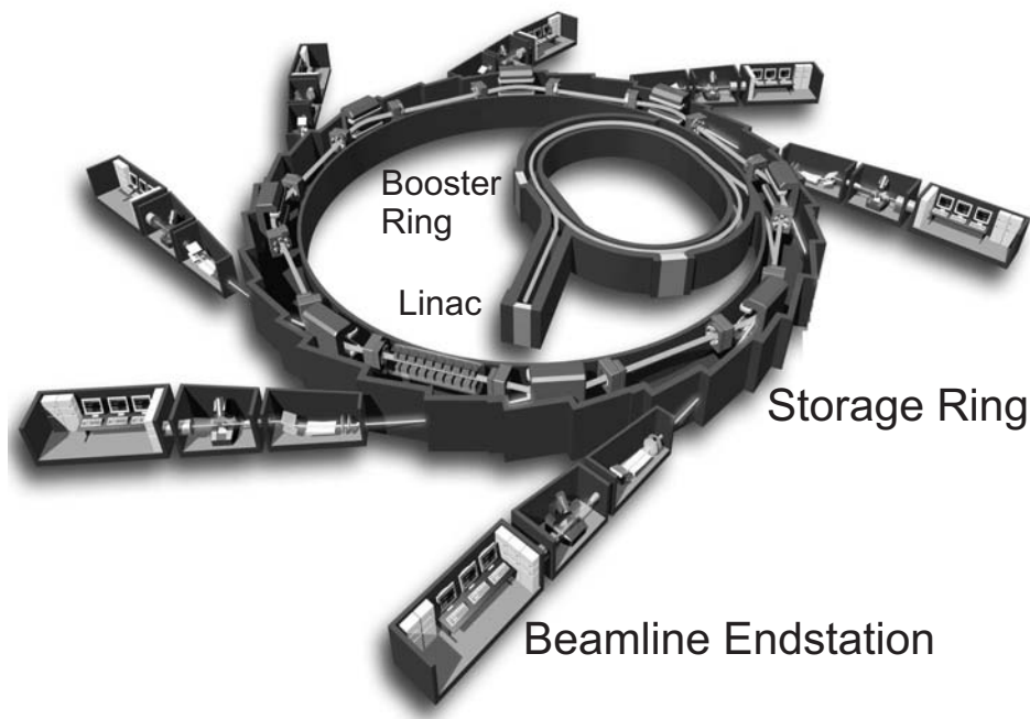
Figure 4.1: Generic scheme of a modern synchrotron storage ring [278]. The key elements of the machine are shown, including the linac, booster and storage rings and the experimental beamline endstations.
