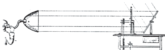
Figure 2.6: Discovery of the photoacoustic effect by Alexander Graham Bell with his photophone.
