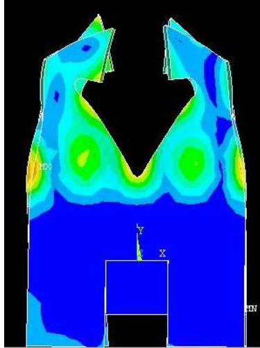
Fig. 7.19: MUM initial structure: 578kHz mode
