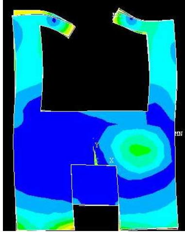
Fig. 7.45: Structure with straight lines: 426kHz mode
