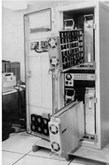
Figure 5. One of the first Interface Message Processor (IMP) of ARPANET connecting UCLA with SRI in August 1969
