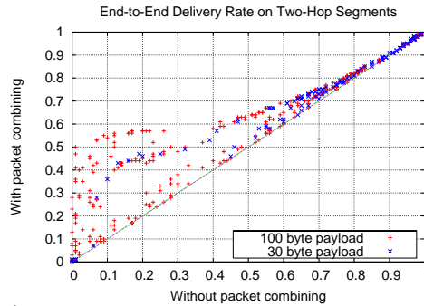
c) Scatter plot comparing end-to-end delivery rate (single-path routing) with and without SPaC.
