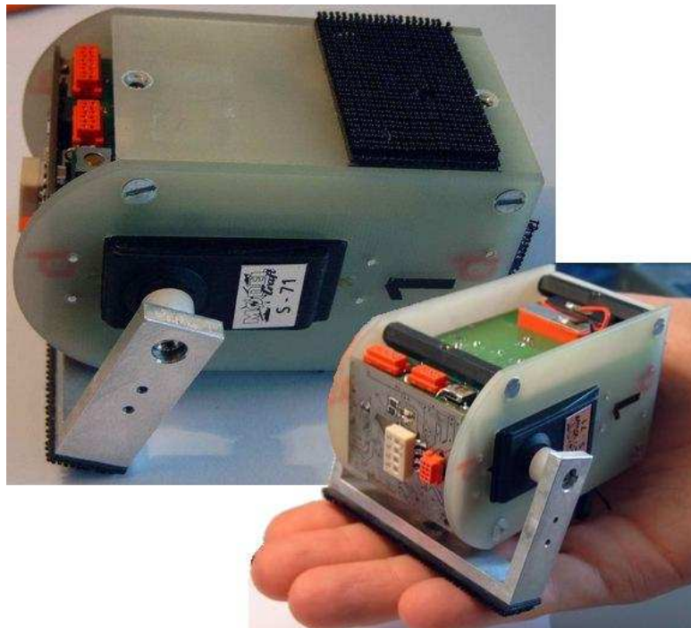
Figure 8.1 YaMoR unit. Unit closed and with open casing
