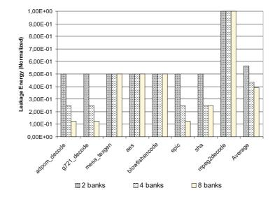
**Fig. 3.** Leakage Energy savings for the three configurations (normalized to non-banked register file)
