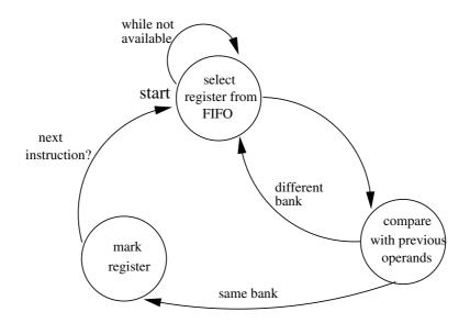
Fig. 2. Register assignment algorithm
