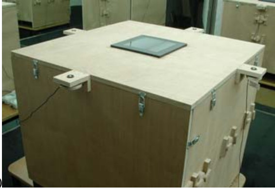
Figure 1. (a) Scale model with the Serraglaze™ sample over the opening surface. (b) Camera positioning system for real sky scenario
