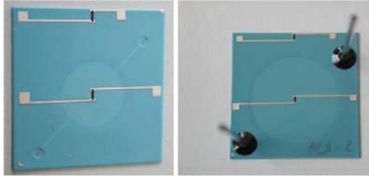
Figure 16. Screen-printed membrane (left). Post-firing followed by completion of inlet and outlet ports.
