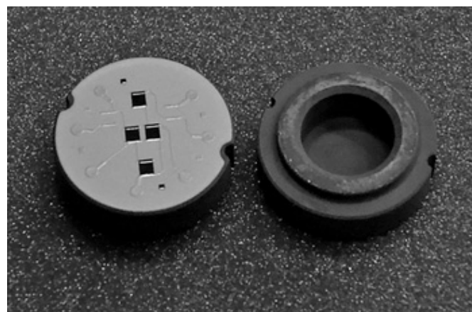
Figure 4: MIM sintered parts (top and bottom)
