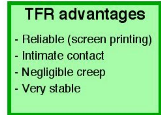
Thick-film resistors possess a **piezoresistive effect**.
