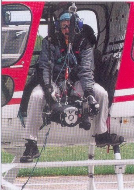
▲ HELIMAP SYSTEM in nadir configuration for downward-looking data capture. It can also be configured to “map” laterally to better capture vertical surfaces.
