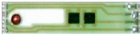
Fig. 1. Top side (side stressed in tension) of force measuring circuit – "MilliNewton" sensor.
