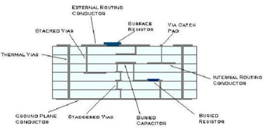
Reliable mechanical, thermal and electrical performance
