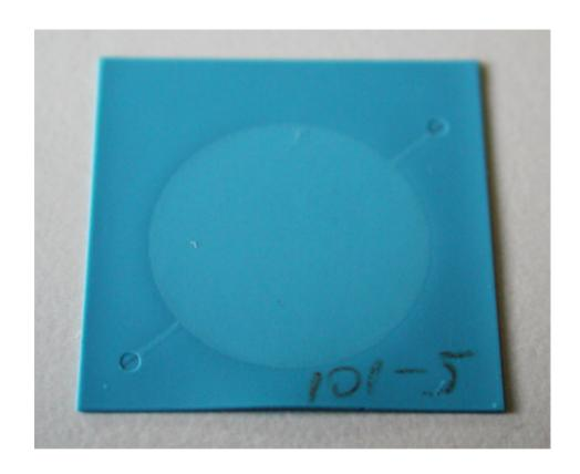
• 15 mm membrane, 40  $\mu$ m thick, 15  $\mu$ m spacing
