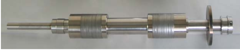
Figure 7.12: Rotor for high temperature AMB.
