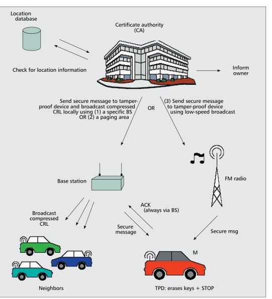
**Figure 5.** *Revocation protocol of the tamper-proof device (RTPD).*
