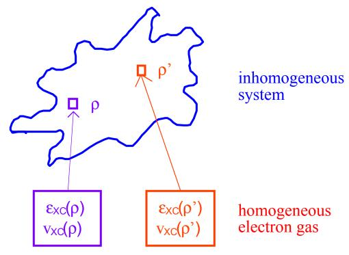
Thus, the averaged exchange potential becomes a function only of  $\rho(r)$ , and the problem of calculating exchange integrals is completely avoided.
