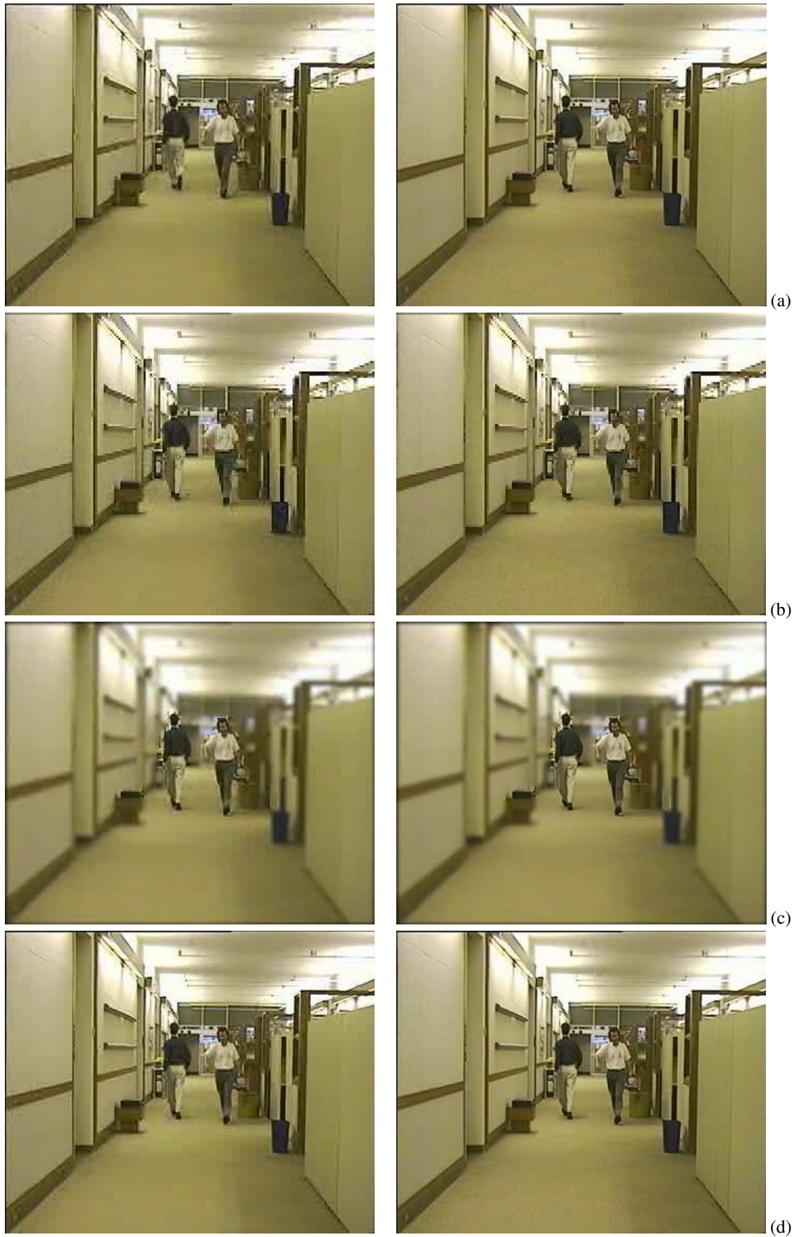
Fig. 4. Frame 190 from Hall monitor for different adaptation strategies. The coding bitrates are: (left column) 176 Kbit/s; (right column) 1000 Kbit/s. The strategies under analysis are: (a) Coded original. (b) Spatial resolution reduction. (c) Lowpass-filtered background. (d) Static background.
