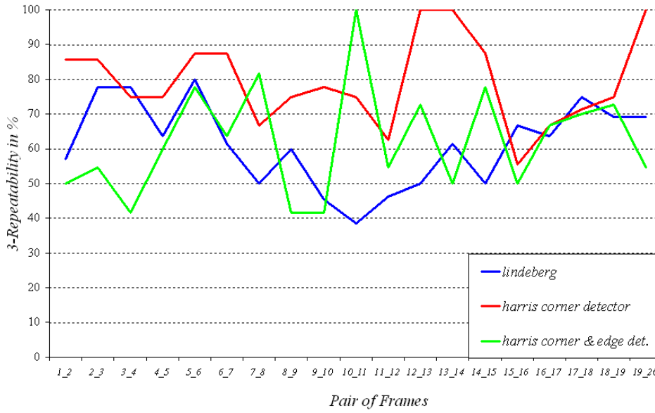
Figure 8.3: 3-repeatability rate with respect to 15-degree rotation during 20 frames (FIVE sequence) for Harris and Lindeberg algorithms.
