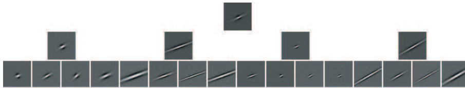
Fig. 13. Bottom part of the tree-structured dictionary, built on gaussian 2-dimensional atoms.
