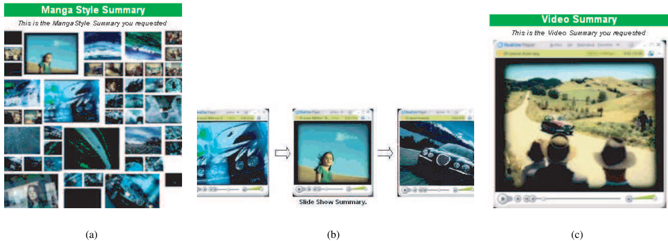
Fig. 4. Three summary representations are supported by PERSEO content preparation software. (a) Pictorial summary ( Manga Style ). (b) Sequential summary using key frames ( Slide Show ). (c) Sequential summary using key sequences ( Video Summary ).
