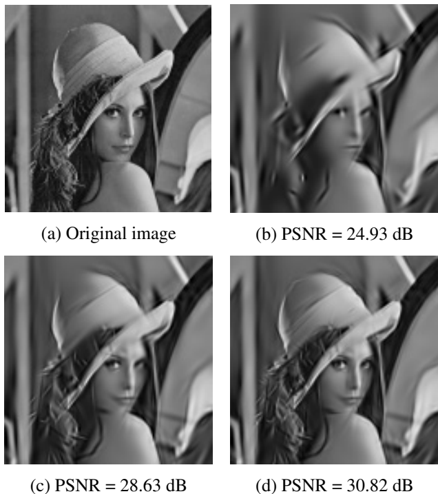
Fig. 2. Lena 128 \times 128 . Original Lena image (a) and its reconstructions using respectively (b) 100, (c) 300 and (d) 500 atoms.
