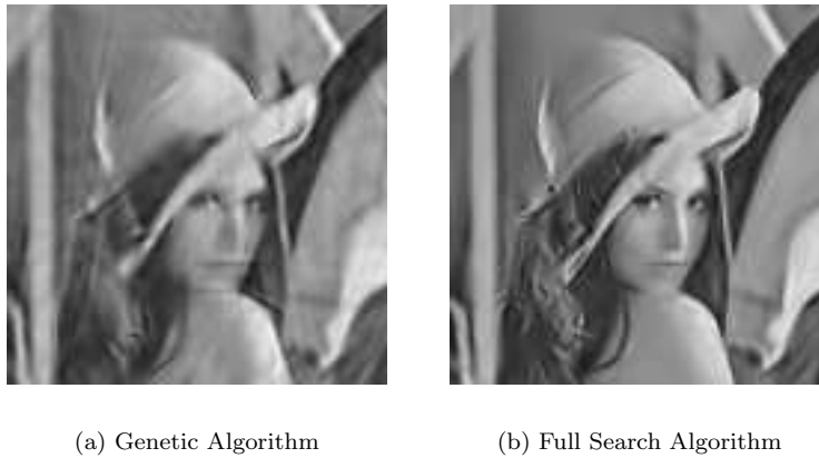
Fig. 5. Visual comparison of lena 128x128 decomposed with MP with 300 coefficients (a) with the Genetic Algorithm and (b) with the Full Search MP.
