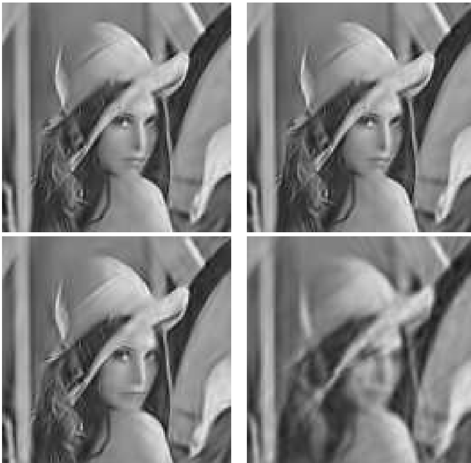
Fig. 12. Visual comparison of the different approximation of lena 128x128 for the amounts of memory of: (from left to right and then up/down) 377 MB (threshold 0), 122 MB (threshold 10 -4 ), 22 MB (threshold 1) and 2.2 MB (threshold 10).
