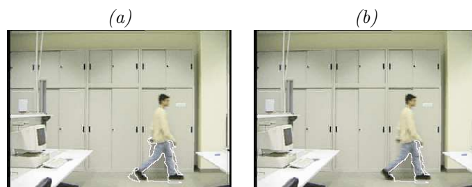
Figure 8. Shadow segmentation results for test sequence Laboratory . (a) Moving cast shadow extraction. (b) Final results after tracking.
