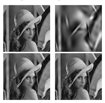
Figure 3. lena image of size 128 × 128 encoded with MP at 1.7bpp (top left), and truncated at 0.1bpp (top right), 0.4 bpp (bottom left), and 0.8 bpp (bottom right).
