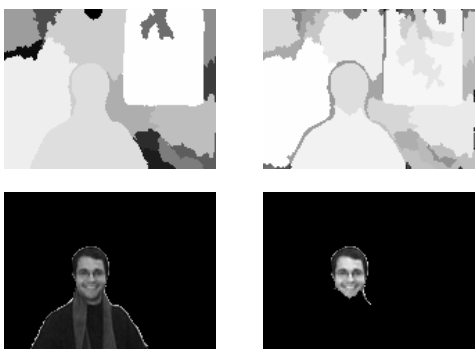
Figure 5: Obtainment of meaningful objects (down) using the Scale-Space segmentation (regions up). Level of segmentation are left: \sigma_n = 30 pixels, right: \sigma_n = 25 pixels.
