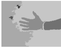
Fig. 17. Segmentation of the image Rosa's hand, using two of the three components: C_i and C_m , with 1.0 and 1000 as weight values respectively.
