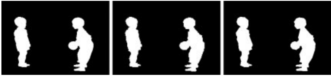
Figure 2: Sequence 'Kids', frame 0. Left: original. Center: quasi-lossless, CAE (avg. 934 bits/frame). Right: quasi-lossless, PPE (avg. 1417 bits/frame).
