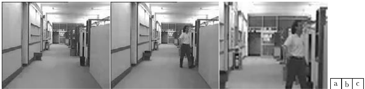
Figure 21: Reconstructed frames of Hall monitor compressed at 48 kbit/sec with the object-oriented configuration. (a) Frame #300 foreground object only, (b) Frame #300 background object only
