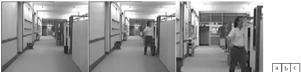
Figure 17: Reconstructed frames of Hall monitor at 48 kbit/sec. (a) Frame #1 (b) Frame #300 (c) Zoom on face area frame #300
