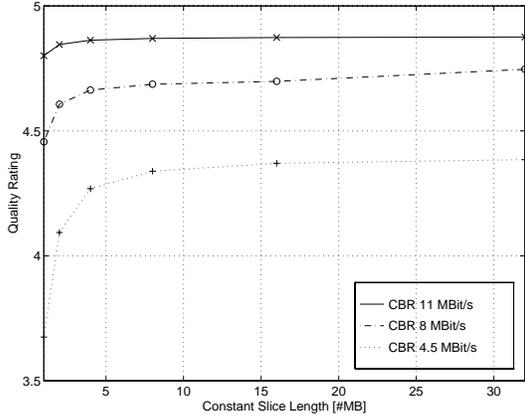
Figure 3: *Perceptual video quality versus number of macroblocks per slice for CBR MPEG-2 encoding. Simulations performed on the Ski sequence at 4.5, 8 and 11 MBits/s.*
