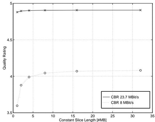
Figure 4: *Perceptual video quality versus number of macroblocks per slice for CBR MPEG-2 encoding. Simulations performed on the BasketBall sequence at 8 and 24 MBits/s.*
