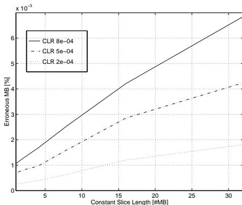
Figure 6: *Number of corrupted macroblocks versus slice length. Simulations performed on the Ski sequence.*
