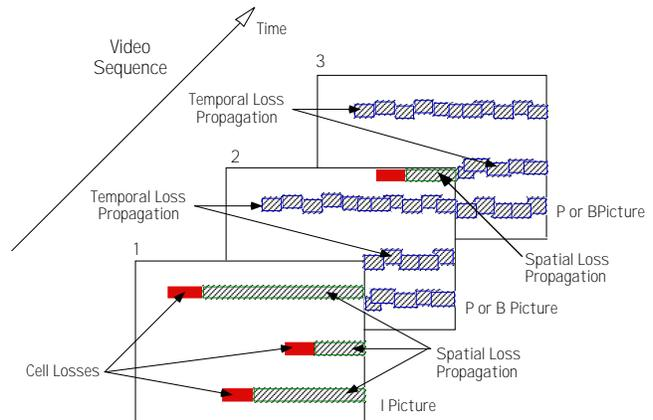
Figure 2: *Data loss propagation in MPEG-2 video streams.*
