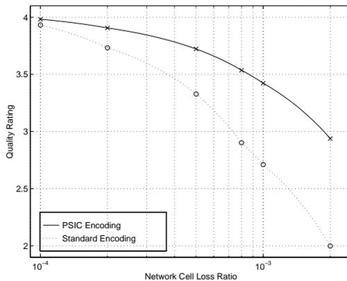
Figure 9: *Perceptual video quality versus the ATM cell loss ratio for both PSIC and fixed-length slice encoding at a CBR of 8 Mbit/s. Simulations performed on the Basketball sequence.*
