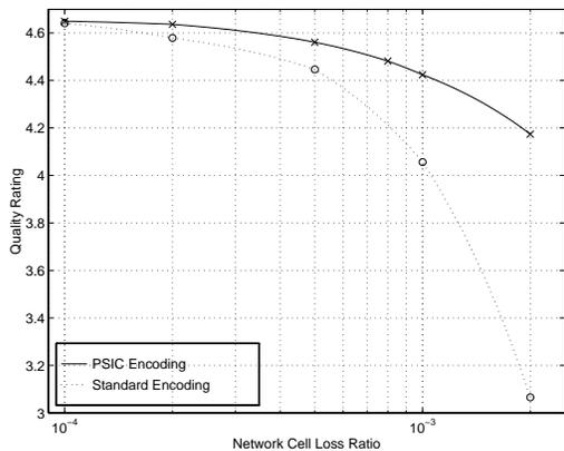
Figure 8: *Perceptual video quality versus the ATM cell loss ratio for both PSIC and fixed-length slice encoding at a CBR of 8 Mbit/s. Simulations performed on the Ski sequence.*
