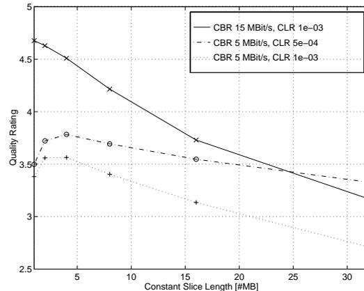
Figure 7: *Video quality versus the slice length for three different couples (constant encoding bit rate, ATM cell loss ratio). Simulations performed on the Ski sequence.*
