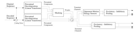
Figure 2: Block diagram of the motion rendition quality metric.
