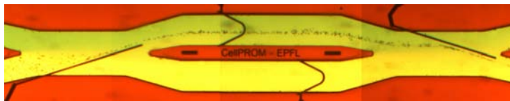
Figure 5.12: Top-view (assembled from video screen-shots) of an improved cell dipping device: Flatter nDEP barriers allow for higher flow speeds, the central separation limits lateral diffusion and additional nDEP traps allow for particle collection in either branch. The common channel is 300\ \mu\text{m} wide, each branch is 200\ \mu\text{m} wide, they are separated over a length of 1.4\ \text{mm} . In the current experiment, 5\ \mu\text{m} diameter yeast cells are deflected from PBS into Trypan Blue dyed buffer.
