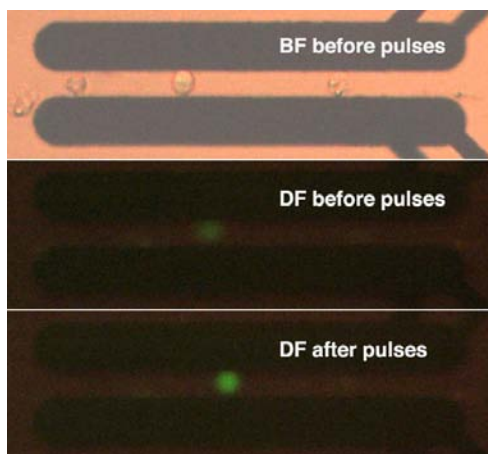
Figure 5.8: Bright- and darkfield top-views of two 25\ \mu\text{m} wide line pair electrodes of 20\ \mu\text{m} height separation and 15\ \mu\text{m} opening. A CHO (chinese hamster ovary) cell is slowly flowing from left to right. The cell is suspended in calcium-rich buffer and pre-loaded with the calcium-dependent fluorescent dye Fluo3 (top, brightfield BF). Initially, the cell is slightly fluorescent due to the intracellular calcium (centre, darkfield DF). Upon the application of 10 rectangular 2.5\ \text{kV/cm} pulses at 100\ \text{kHz} , the cell membrane becomes permeable to the extracellular calcium diffusing into the cell and increasing the fluorescence within a fraction of a second (bottom, DF).
