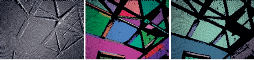
Figure 4.9: A part of a scanned scene showing the ceiling structure at our lab. Note that the cross beams shown in the raw scan on the left break up the single planar segment describing the ceiling into several subsegments depicted in different colors in the middle image. The right image shows the result of the post-processing step, where the several segments of the ceiling (see middle image) have been fused to a single region.
