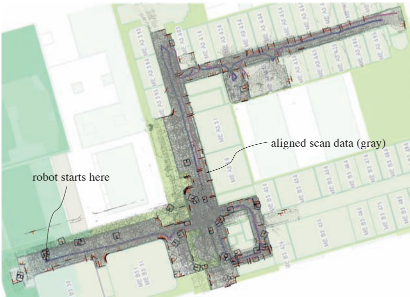
Figure 6.11: In this experiment, the complete corridor of our lab was reconstructed. The robot travelled 140m and took 90 3D scans in a stop-and-go manner. The resulting map is visualized as aligned raw data (gray) overlaid onto a building map for visual comparison. The total number of found planar features is 244, see also figure 6.12.
