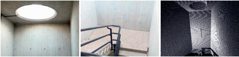
Figure 2.3: The scene chosen for calibration is the top floor of the stairway leading to our lab. It features a cuboidal structure which is easy to measure by hand. The right-most image shows a 3D scan of the scene, whereas the other two are photos. Note that the hole in the roof can be found again in figure 2.4.
