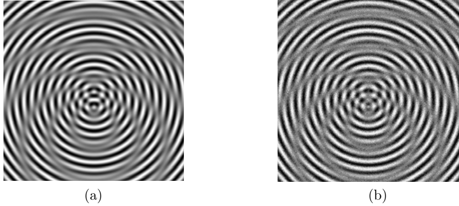
Fig. 1.2: Moiré fringes ( 512 \times 512 pixels) corresponding to Eq. (1.2). In (a) the random phases \Phi_{ran1} = \Phi_{ran2} = 0 , while in (b) \varphi_1 and \varphi_2 are assumed to be random.
