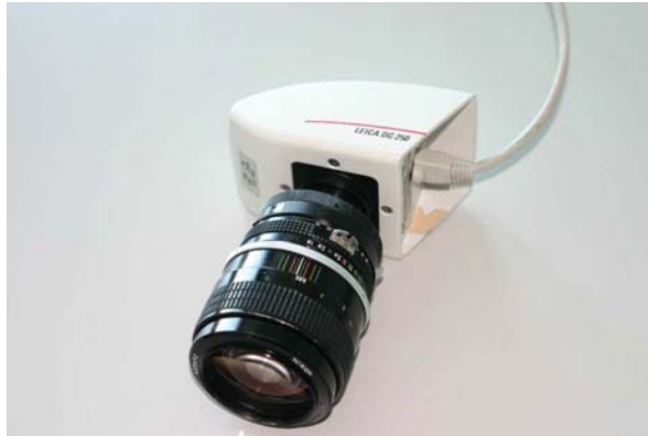
Figure 4.1: Leica DC250 digital camera with a Nikon 85mm optical system used in the first experiment.
