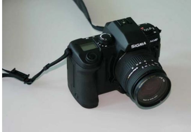
Figure 4.9: Sigma SD10 digital camera with a Sigma 18-50 mm lens used in the second experiment.
