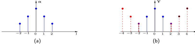
Figure 2.8: Signal spectrum before (a) and after sampling (b), for L = 5 and N = 4 . The base spectrum (—) and aliased spectrum (— —) overlap for the first and last spectral component, corresponding to the first and fifth column in (2.36).
