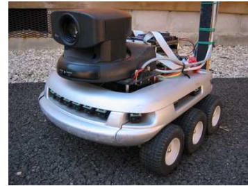
Fig. 2. The Koala mobile robot by K-Team S.A. with a pan/tilt camera in an outdoor environment.
