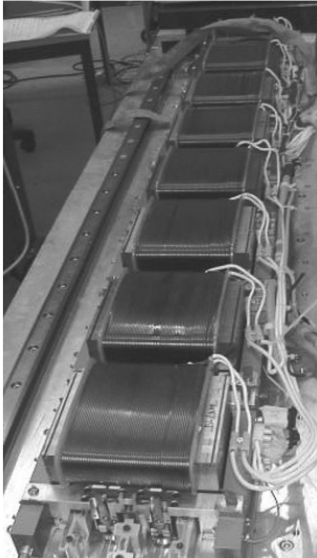
Figure 4.56: Four phases TFM prototype composed by eight motor modules.
