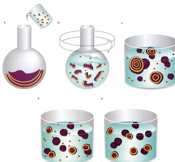
Figure 4.5: Thin-film hydration approach to produce lipid vesicles. Schematic representation of MLV preparation (a-c) through agitation of the flask; relatively homogeneous population of unilamellar vesicles can be prepared by following slow swelling process (classical swelling) as shown in (d). This approach would result with a high percentage of GUVs [145]; (e) a dialyzed preparation of (d) will ensure that all non-entrapped molecules are decanted away (adapted from [72]).
