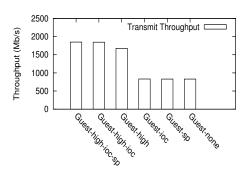
Figure 10: Transmit performance with writes
