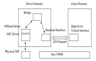
Figure 2: New I/O Architecture
