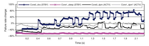
Fig. 9. Comparison of standby-parallel (STBY) and active parallel (ACTV).
