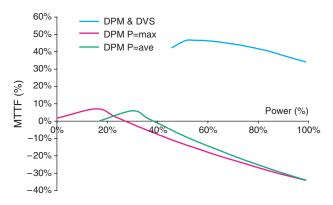
Fig. 11. Power and MTTF improvement due to DVS and DPM on XScale.
