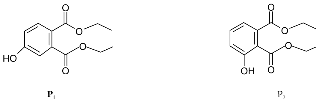
Figure 2. 5: Molecular structure of two by-products of photodegradation of the DEP: ( P_1 ) absorbs maximum at 256 nm and ( P_2 ) absorbs at 302 nm. (Mailhot et al., 2002). In our work, we assume that the by-products observed with maximum absorption at 253.4 nm and 301.3 nm are the same as P_1 and P_2 respectively. The slight differences of data (253.4 # 256 nm) and (301.3 # 302 nm) could be due to the difference of the analytical procedures or devices.
