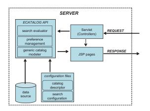
Figure 6: The architecture of ECATALOG, the generic preference based search tool.
