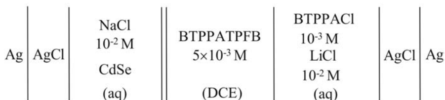
Figure 5.3 Schematic composition of the electrochemical cell.
