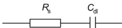
Figure 2.5 Equivalent circuit for the liquid|liquid interface in the absence of Faradaic process.
