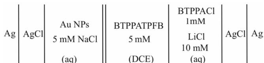
Figure 4.1 Schematic representation of the electrochemical cell employed for the measurements in Chapter 4.
