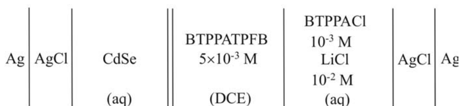
Figure 5.13 Schematic composition of the electrochemical cell.
