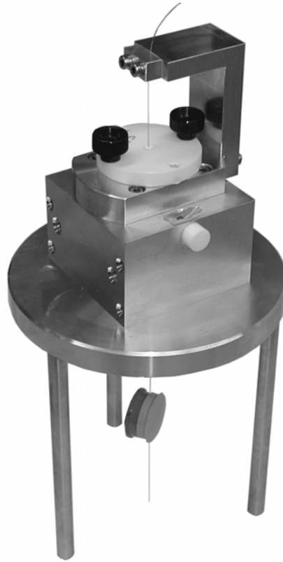
Figure 4.6: Mould used to prepare the cylindrical specimen in the "Vertical configuration".
