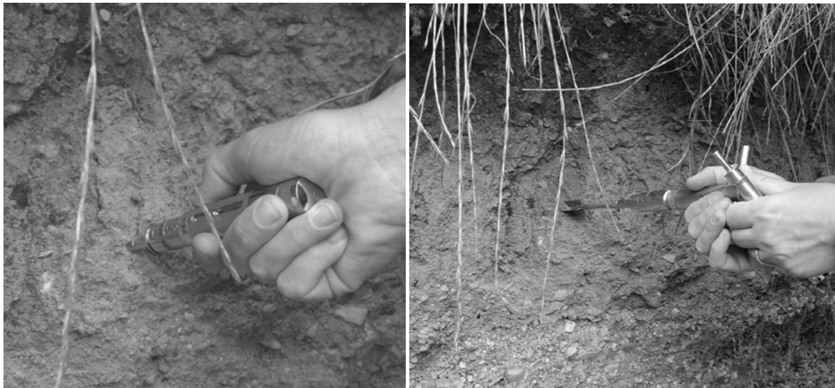
Figure 4.34. Pocket penetrometer (left) and shear vane (right) used during the Lower Venoge bank investigations
