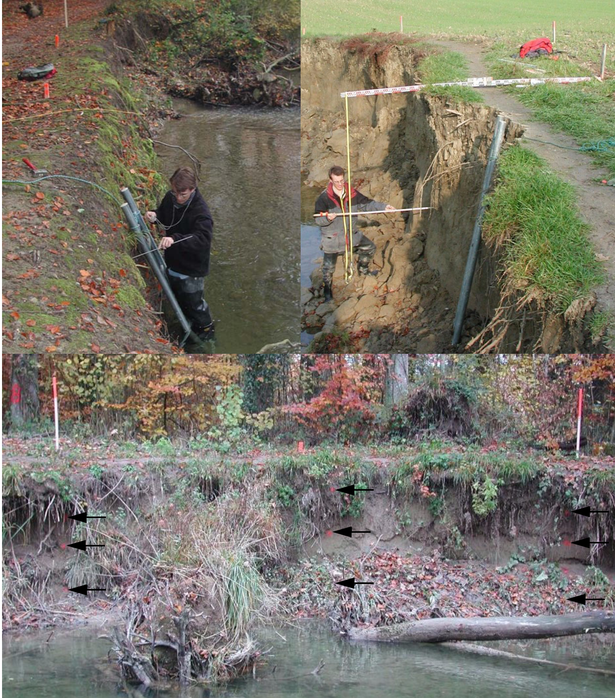
Figure 4.5. Erosion monitoring on the Lower Venoge River. Bottom shows a small monitoring bend (pin locations marked by arrows). Upper left shows the pin installation. Upper right shows the bank profiler.
