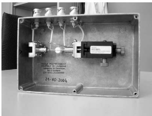
Figure 4.2: The sample holder, with the five terminal configuration, for low capacity measurements made in our laboratory (left); the stray capacity of the 5-terminal setup as a function of frequency - the accuracy of the configuration can be estimated to \pm 1fF (right).
